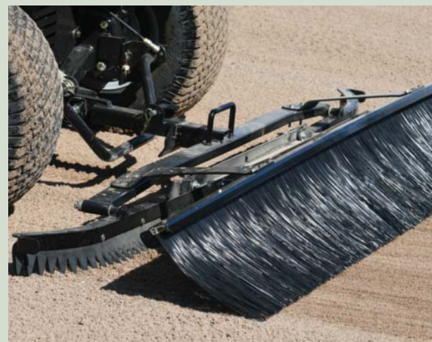
45-511 serrated rubber rake with optional finish brush
